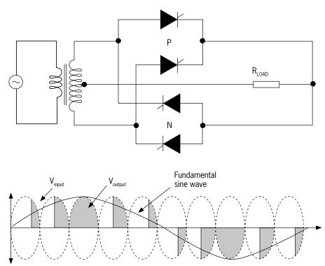
Each converter is a bi-phase half-wave connection; the positive group labelled P and the negative group (for reverse current) labelled N.
