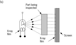
The fluorescent screen is replaced by a film holder containing a sheet of X-ray-sensitive film. The film is positioned with the object being examined between the film and the X-ray tube. After exposure, the film is developed in the usual method of processing photographic film and after being dried, it is viewed by placing it on a brightly lighted sheet of glass in the same manner as done with medical X-ray films.
