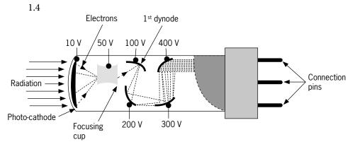
A photo-multiplier uses the principle of fluorescence, where radiation with energies equal to or greater than those of visible photons causes certain phosphorous materials to emit a visible glow when radiation energy excites the phosphorous materials.
