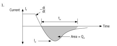
Given a forward diode or thyristor current  $I_{p}$  which is turned off at a given  $\frac{di}{dt}$  rate, the current will go into reverse until the carrier storage charge  $Q_{rr}$  is recovered. At defined values of  $I_{p}$  and  $\frac{di}{dt}$ , a particular device will have rated values of  $Q_{rr}$  (the reverse recovery charge) associated with a reverse recovery time  $t_{rr}$  and a reverse recovery current  $I_{rr}$ .
