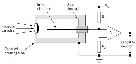
Radiation moves about randomly outside the detector tube. Some of the radiation enters the window at the end of the tube. When radiation collides with gas molecules in the tube, it causes ionisation: some of the gas molecules are turned into positive ions and electrons.
