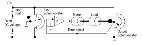
The input potentiometer is adjusted to the required setting (set point). This sets up a difference signal voltage across the input of the amplifier. The error voltage is amplified and drives the servo motor. The shaft of the motor is mechanically coupled to the load and output potentiometer, which is displaced at the same angular displacement as the motor shaft. A new voltage setting is thereby produced on the output potentiometer.
