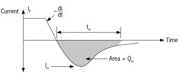
Given a forward diode or thyristor current  $I_{p}$ , which is turned off at a given  $\frac{di}{dt}$  rate, the current will go into reverse until the carrier storage charge  $Q_{rr}$  is recovered. At defined values of  $I_{p}$  and  $\frac{di}{dt}$ , a particular device will have rated values of  $Q_{rr}$  (the reverse recovery charge) associated with a reverse recovery time  $t_{rr}$  and a reverse recovery current  $I_{rr}$ .
