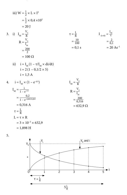
The time constant of an RL circuit is the time taken for the circuit to reach steady-state conditions after a disturbance, assuming a constant rate of change in charging or discharging current.
