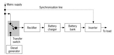
In the forward system, the load is supplied from the mains line via the charger, battery and inverter. In the event of a power failure, the static transfer switch automatically transfers from the AC mains supply to the output of the diesel generator. When power is restored, the load is transferred back to the mains supply via the inverter and the diesel generator is disconnected.
