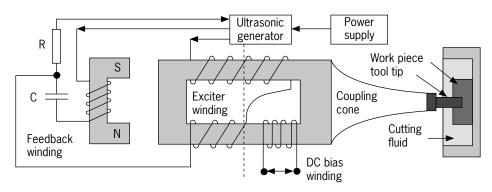
The machine consists of a magnetostrictive core that is clamped at the nodal line. At one end of the core, an exponential cone is attached, which carries the cutting tip. The other end of the core is coupled to the feedback circuit in order to sustain oscillations.
