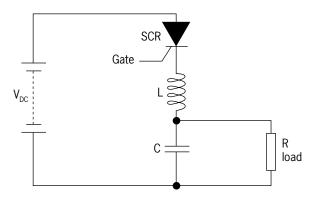
The self-oscillating property of a capacitor-inductor combination can be utilised to turn off the load thyristor at a given time after turn-on without the need for a second or auxiliary thyristor. The series resonant circuit must be underdamped for the thyristor current to attempt to reverse and turn-off to take place.
