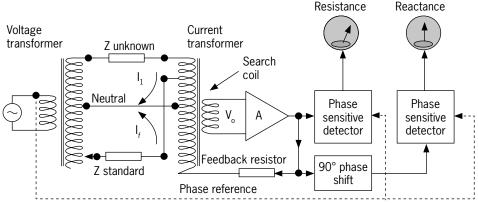
The transformer ratio arm bridge utilises a current balancing technique. One winding on a transformer core receives alternating current  $(I_1)$  produced by a known voltage and unknown impedance. A second core winding is driven by a balancing current  $(I_f)$  produced by a known variable voltage and known standards of resistance and capacitance. A further core winding acts as a search coil to allow determination of a null in the core flux.
