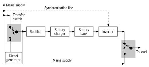
A combination of the forward and reverse system effectively gives double protection in the event of power or inverter failure.
