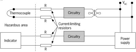
Current-limiting resistors are commonly used as a form of series protection in restricting the amount of current reaching hazardous areas.
