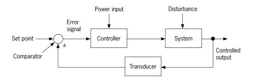
A closed-loop system is one that senses the output, compares the output against a desired condition and then corrects the system to achieve the desired output without the aid of a human operator.
