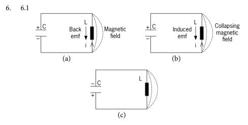
Assuming the capacitor C is to be charged to the polarities indicated in (a) and is then connected to the inductor, the energy stored in capacitor C will discharge trough inductor L and will set up a magnetic field around the inductor, as illustrated in (a).
