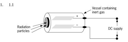
The ionisation chamber essentially consists of a closed vessel containing a gas and is equipped with two electrodes at different electrical potentials. The electrodes, depending on the type of instrument, may consist of parallel plates or coaxial cylinders, or the walls of the chamber may act as one electrode and a rod inside the chamber acts as the other.
