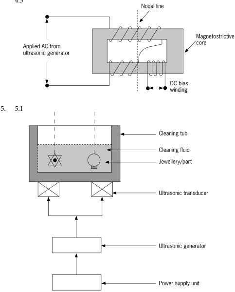
5.2 The cleaning apparatus consists of a cleaning tub with ultrasonic transducers attached to the sides and/or bottom of the tub and is normally attached to the outside of the tub.
