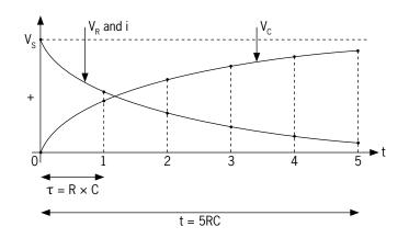
The time constant of an energy-storing circuit may be defined as the time taken for the circuit to reach steady-state conditions after a disturbance, assuming a constant rate of change in the charging or discharging current.
