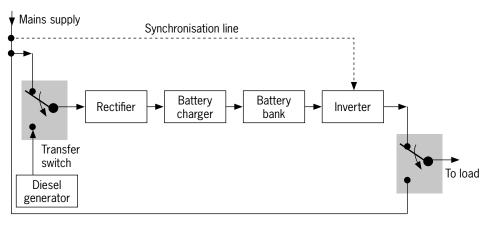
In the reverse system, the load is supplied from the inverter and is only transferred to the mains supply as a result of an inverter failure.
