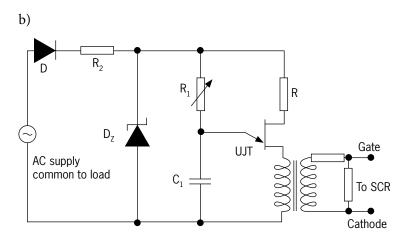
Both circuits are supplied from an AC source that is clipped by the Zener diode  $D_z$  to give a level voltage to the  $R_1C_1$  series circuit. Resistor  $R_2$  drops the voltage difference between the supply and the Zener diode. In both circuits, the voltage on capacitor  $C_1$  will rise exponentially at a rate determined by the value of resistor  $R_1$ .
