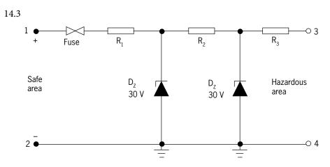
It is so designed to ensure that when the mains supply is applied to terminal 1 (zone 2 area), the voltage and current at terminal 3 (zone 0 area) are safe.
